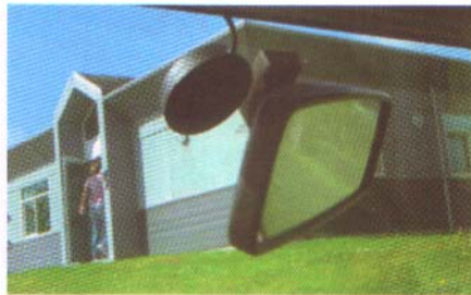
↑ The GPS antenna on the car's windshield
