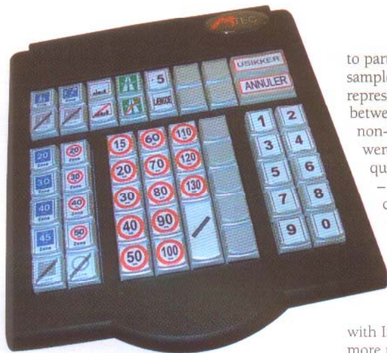
↑ The GPS logger with special keyboard
