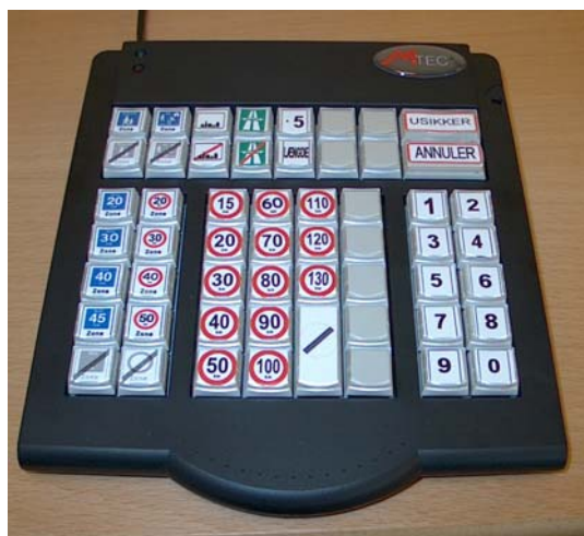
Figure 4 — Special designed keyboard for registration speed sign
